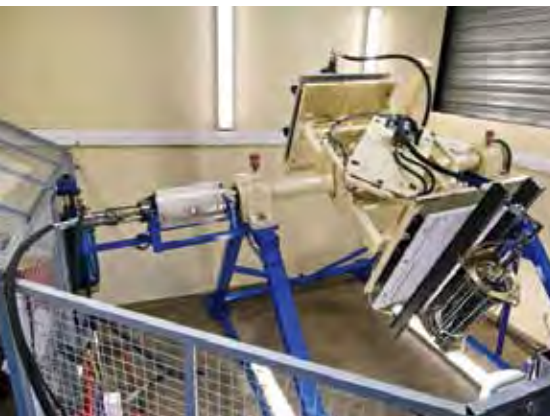
Accumulator test bench for wind turbine application.
