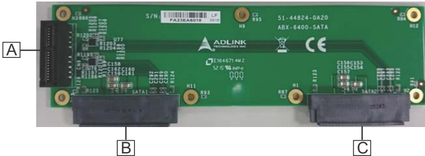
Figure 1-18: SATA Board PCB (Top)
