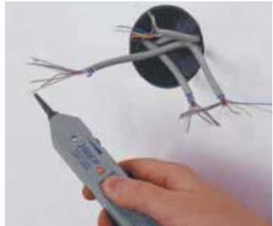
Simply connect the transmitter and cables can be quickly detected.
