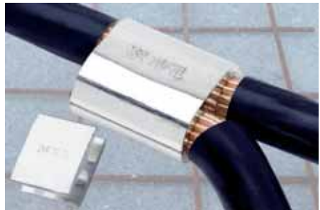
The H-clamps in our range are lightning current tested to EN 50164-1 Class H (100 kA 10/350 \mu s).
