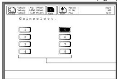
Set the gain level based on the waveform amplitude. The higher you set the gain, the larger the amplitude will be.
