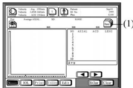
Set the measuring mode by touching the **Mode** button (1). Successive presses of the button scroll through the options. There are two automatic modes and one manual mode.
