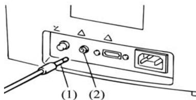
Insert the power plug (1) for the chinrest fixation lamp into the terminal (2) labeled "FIX LIGHT" on the back of the AL-2000.
