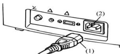
Plug the power cord connector (1) into the terminal (2) on the back of the AL-2000
