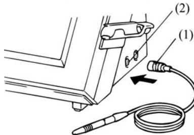
Plug the biometry probe connector (1) into the terminal (2) labeled BIO on the right side of the instrument. When it is properly inserted, you will hear it click.
