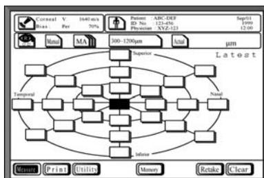
1. Apply the pachymetry probe perpendicular to the cornea at the location corresponding to the reverse-highlighted location on the map array.
