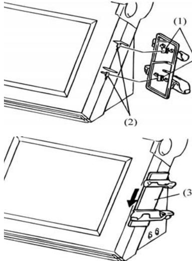
1. Insert the protruding rectangular tabs (1) on the probe holder into the holes (2) on the right side of the instrument.
