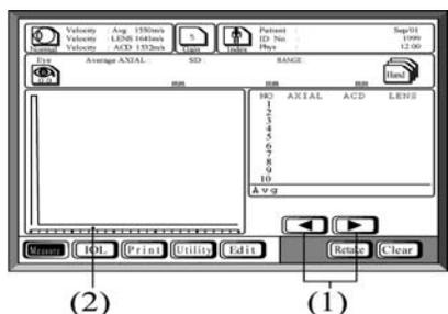
In the event that a spike occurs between the back of the lens and the retina (e.g., due to a vitreous hemorrhage), manually reposition the retinal cursor (2) by pressing the retinal cursor shift keys (1).
