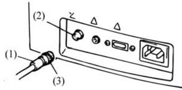
1. Plug the connector (1) for the foot switch to the terminal (2) labeled FOOT SW on the back of the AL-2000. Line up the slot of the connector with the tab on the terminal.
