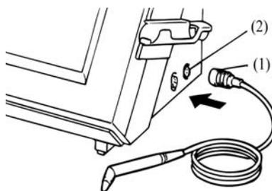
Plug the pachymetry probe connector (1) into the terminal (2) labeled PACHY on the right side of the instrument. When it is properly inserted, you will hear it click.
