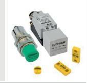
Inductive ident systems Inductive ident systems are used for the non-contact identification of tools, workpiece carriers, pallets, containers and vehicles in the entire logistics sector. The read/write data carriers function completely wear-free and without batteries using inductive coupling.
