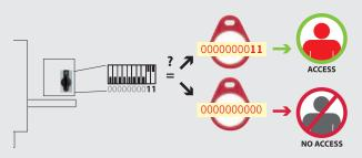
The Electronic-Key adapter and Electronic-Key are separately parameterized, with values which have to match. Parameter assignment to the Electronic-Key adapter is performed very simply through DIP switches.
