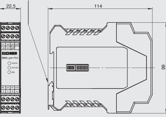
Dimension drawing Electronic-Key adapter EKS Front hook modular FHM
